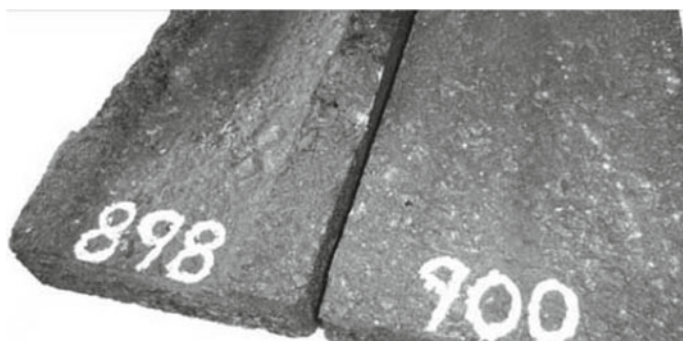
Fig. 2 Two plates after being submitted to the traffic simulator Source Greca Asfaltos [7]
