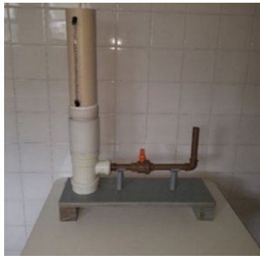
Fig. 4 Variable charge permeameter used. (Color figure online)
