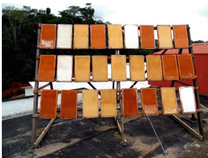
Fig. 4 Result of the weathering test of paint samples after one year of exposure. (Color figure online)
