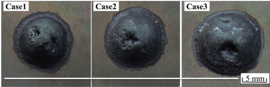
Fig. 7 Macroscopic feature of liquid phase in the fluidity tests. (Color figure online)
