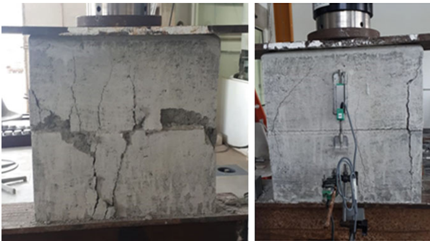
Fig. 3 Rupture mode of the prisms with full bedding type. (Color figure online)
