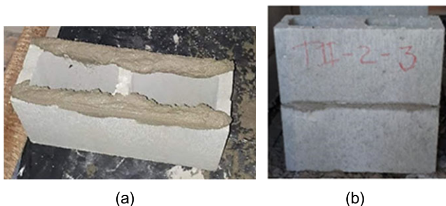
Fig. 2 Construction of the prisms: a detail of the face shell bedding type b constructed prism. (Color figure online)
