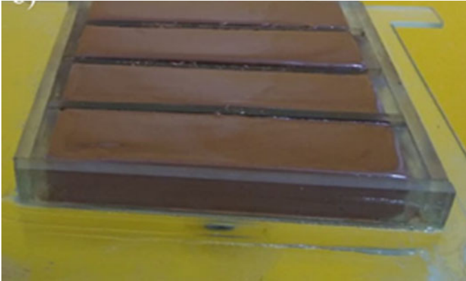
Fig. 1 Specimens molded in an acrylic container. (Color figure online)
