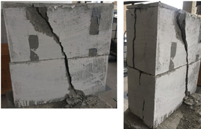
Fig. 3 Rupture mode of the prisms with face shell bedding type. (Color figure online)
