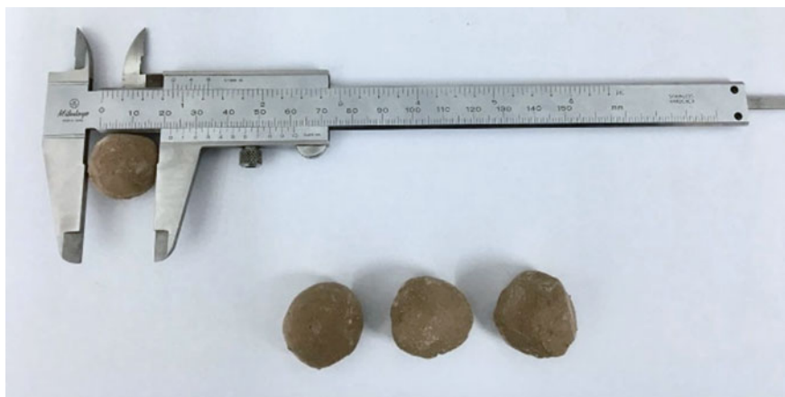
Fig. 1 Molded pellets with diameter of 1–2 cm. (Color figure online)
