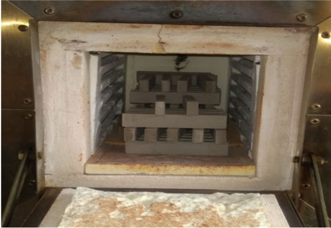
Fig. 3 Ceramic parts in the firing phase in an electronic muffle. (Color figure online)
