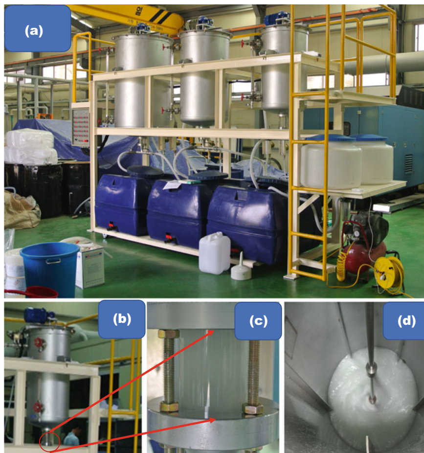
Fig. 3 Demonstration plant view a complete 3-stage batch scale operated plant, b typical agitation and phase separation unit, c visual apparatus unit for phase separation observation, and d inside view of baffle mixture tank. (Color figure online)
