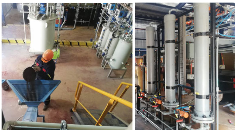
Fig. 7 Left: Leaching Pilot unit at MYTILINEOS; Right: II–VI SIR Pilot unit installed at MYTILINEOS. (Color figure online)
