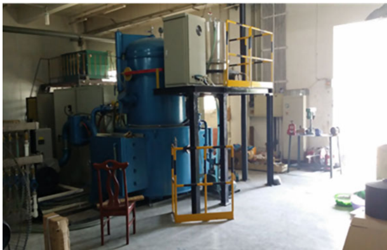
Fig. 1 120 kW continuous reduction of lithium test furnace. (Color figure online)
