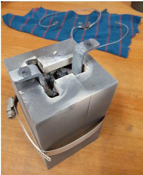
Fig. 2 Lantern Reactor after cooling following 3 min resistance heating triggering a reaction with aluminothermic sodium sulfate reactant ( Courtesy Powerball Technology ) (Color figure online)
