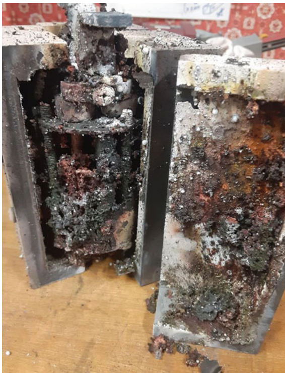
Fig. 4 Lantern reactor with products. Products are powdery substances easily scraped out into containers (Courtesy Powerball Technology) (Color figure online)
