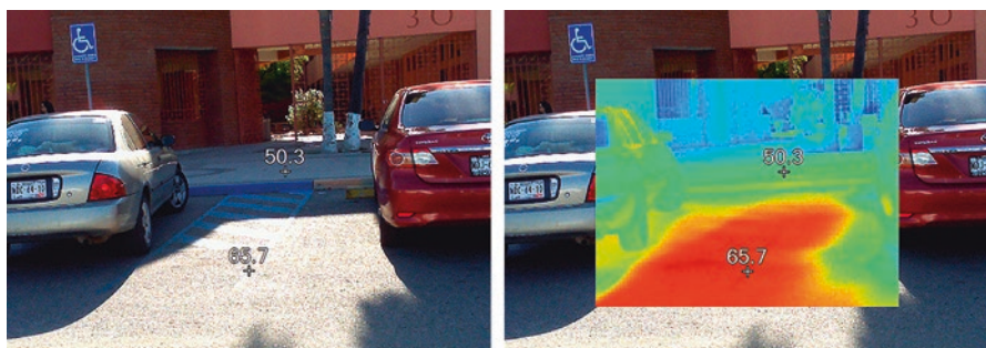
Fig. 8.13 Visible (left) and infrared photography (right) of case 3. False color scale is 30–70 °C
