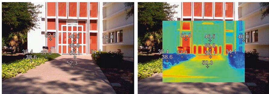
Fig. 8.11 Visible (left) and infrared photography (right) of case 1. False color scale is 30–70 °C
