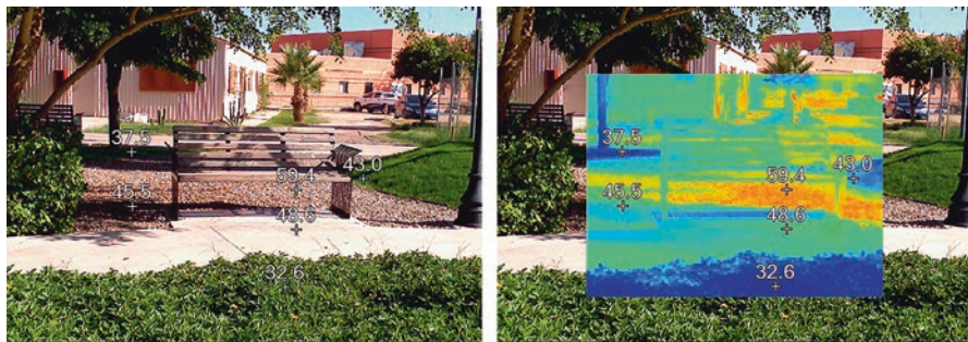
Fig. 8.12 Visible (left) and infrared photography (right) of case 2. False color scale is 30–70 °C
