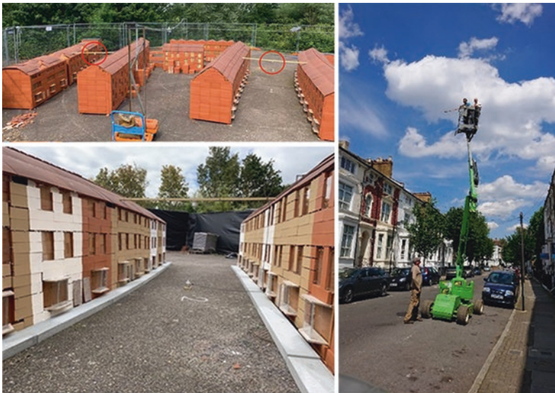
Fig. 5.17 1:10 scale model constructed at the University of Kent and full-scale spot measurements at the case study area in London
