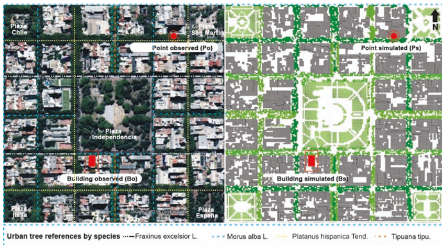
Fig. 22.1 Aerial view of the studied area and numerical model configuration with ENVI-met 3.1. Location of point observed (Po) and simulated (Ps), and building observed (Bo) and simulated (Bs). Description of urban trees. (Source: Own elaboration 2019)
