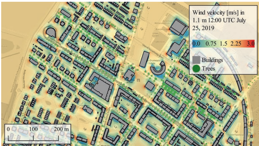
Fig. 16.8 Diagnostic wind speed under prevailing boundary conditions of 3 m/s and a wind direction of 350°, calculated by SkyHelios. Wind speed and wind direction are calculated for 12:00 UTC on July 25, 2019
