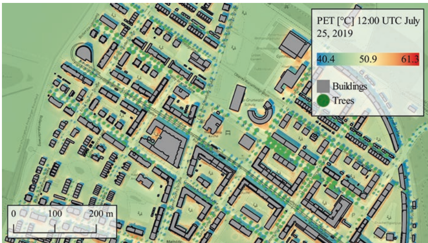
Fig. 16.9 SkyHelios can assess human thermal comfort in terms of the physiologically equivalent temperature (PET). PET can be computed spatially resolved with variable spatial resolution for different urban environments by SkyHelios. PET is calculated for 12:00 UTC on July 25, 2019
