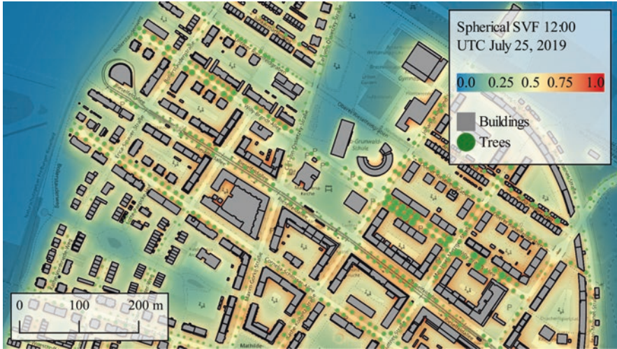
Fig. 16.6 The obstruction of the upper hemisphere by the urban morphology (e.g., buildings and trees) can be calculated by SkyHelios in terms of spherical and planar sky view factor (SVF). SVF can be computed spatially resolved with variable resolution for different urban environments due to preexisting urban city models. This SVF is calculated for 12:00 UTC on July 25, 2019, in 1 m height
