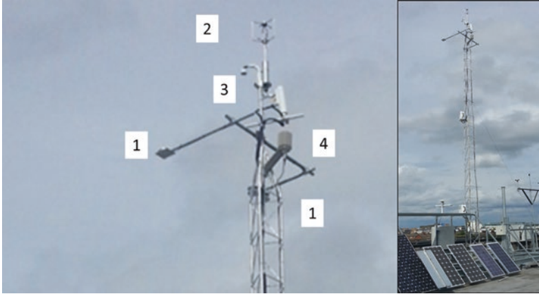
Fig. 3.4 Eddy covariance instrument platform located in a mid-rise neighbourhood (LCZ 2) in Dublin (Ireland). The instruments shown are net radiometers (1), three-dimensional sonic anemometer (2), gas analyser (3) and temperature/humidity sensor (4). These instruments are mounted at height well above the surrounding urban landscape
