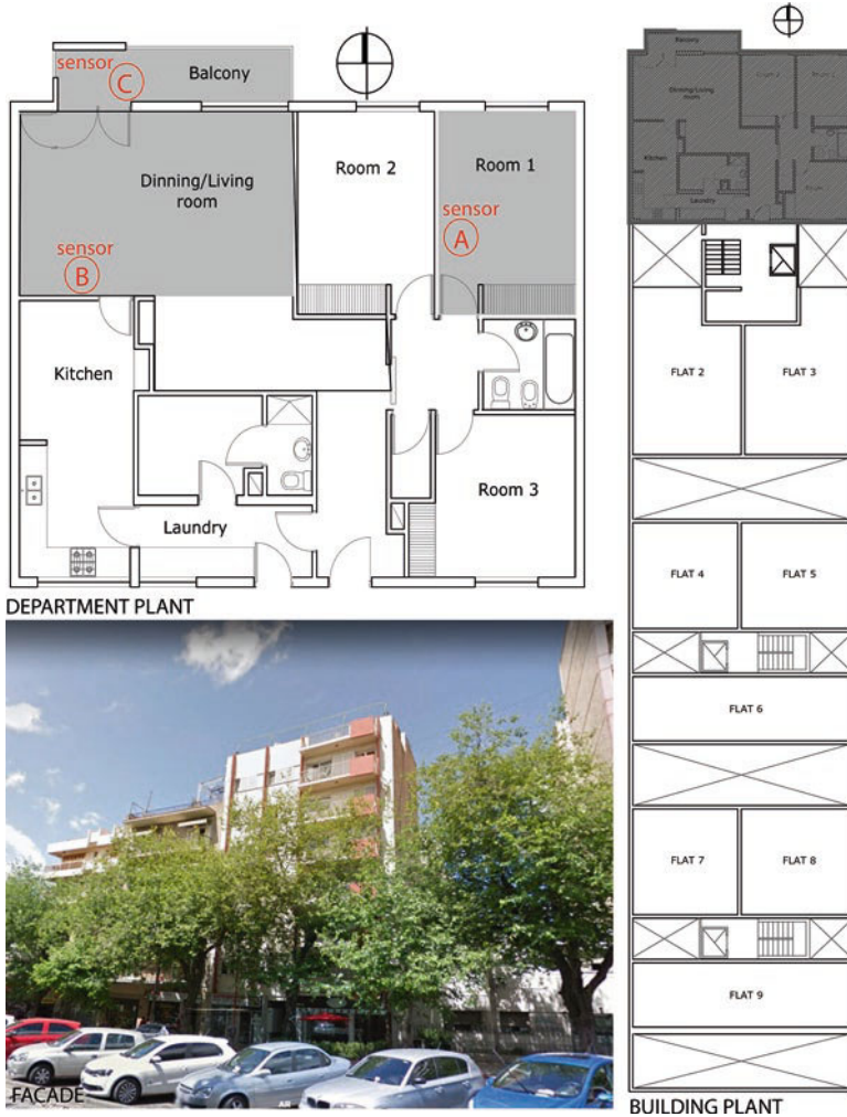
Fig. 22.3 Image and plan of the selected building. Plan of the monitored housing unit in three different heights: first floor, fifth floor, and eighth floor (upper level). (Source: Own elaboration 2019)
