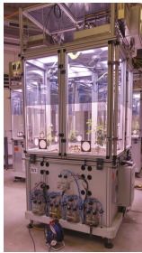
Fig. 2. An EcoUnit from the Ecotron system.
