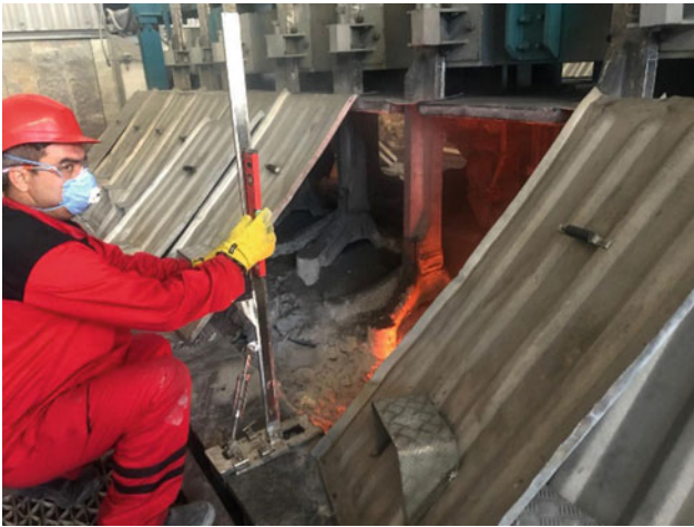
Fig. 3 Ledge measurement at ALRO. (Color figure online)
