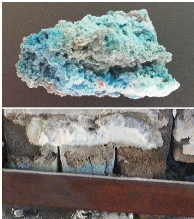
Fig. 1 Samples of the mineral diaoyudaoite removed from a modern cell. Upper from ledge sample and lower on sidewall end of anode butt. (Color figure online)
