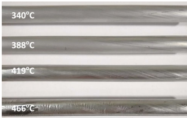
Fig. 2 Surface appearance for AA 7075 tubes extruded by ShAPE at 7.4 m/min
