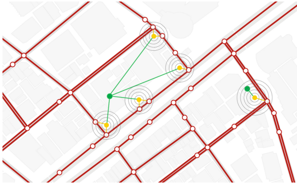
Fig. 3. Stations (green) are connected to exits (yellow) which are in turn connected to their surrounding road nodes (red). Using increasingly larger circles ensures at least one connection, but may also include additional road nodes within a similar distance (Color figure online).
