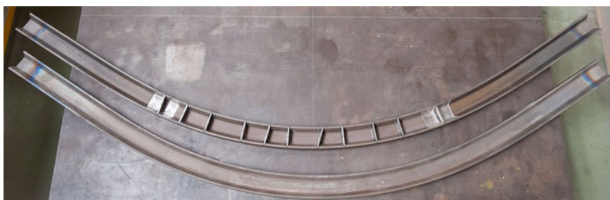
Fig. 13 Combination of extrusion (“U” profile), Hot Stretch Forming and LFW for a door frame demonstrator. (Color figure online)
