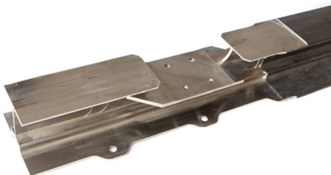
Fig. 12 Combination of extrusion (“H” profile) and LFW for a seat track demonstrator. (Color figure online)
