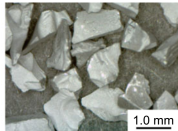
(b) d_{WC-Co} > 0.71 \text{ mm} , irregular shape
