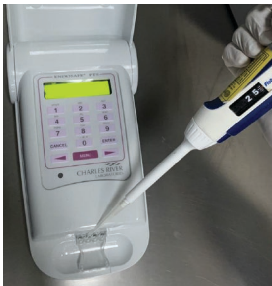
Fig. 3.16 The Charles River Endosafe®-PTS™ System, an FDA-approved endotoxin system. A point-of-use and rapid portable system that provides quantitative LAL results in a
