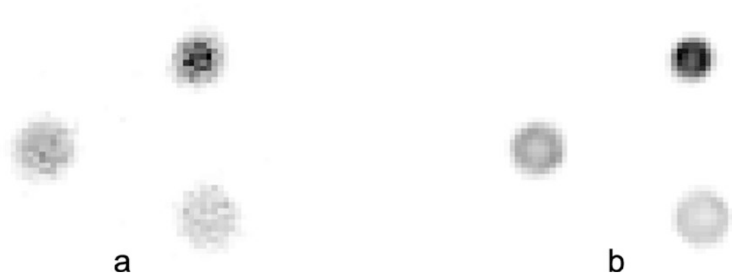
Fig. 18.13 Figure shows the artefacts introduced by the collimator-response compensation. Left image (a) shows three spheres reconstructed with scatter and attenuation compensation. Right figure (b) shows the same recon-
