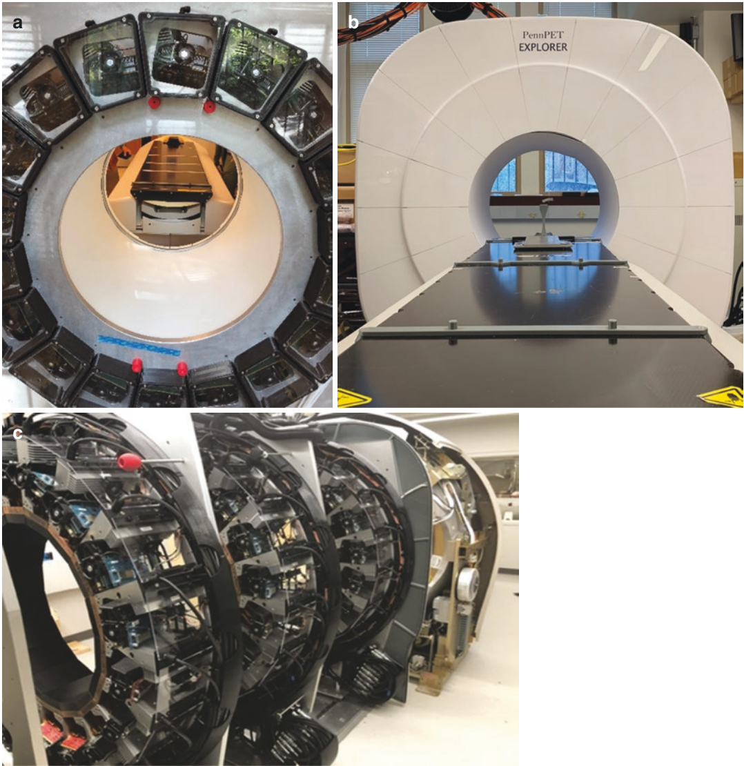
Fig. 12.7 Photographs of the PennPET Explorer showing the (a) axial extent, (b) table of the patient couch along with (c) general view of internal anatomy demonstrating the 3 ring design of the scanner. Many thanks to
