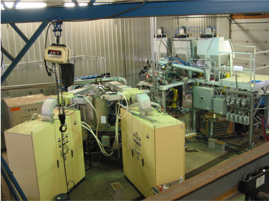
Fig. 4 A top view of MW/PA-RHF and material feeding system. (Color figure online)
