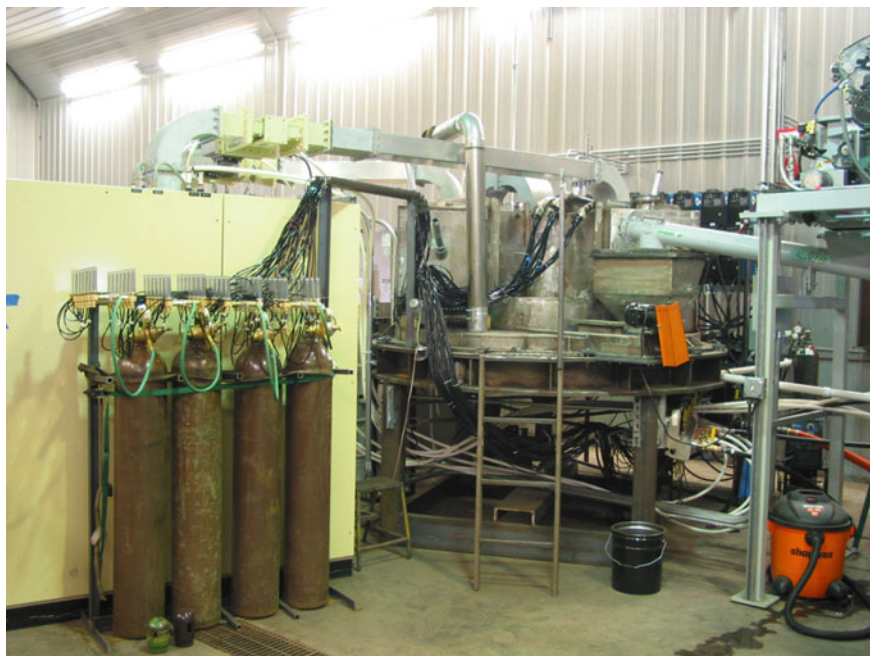
Fig. 6 Gas station to provide gas for the 52 electric arcing torches. (Color figure online)
