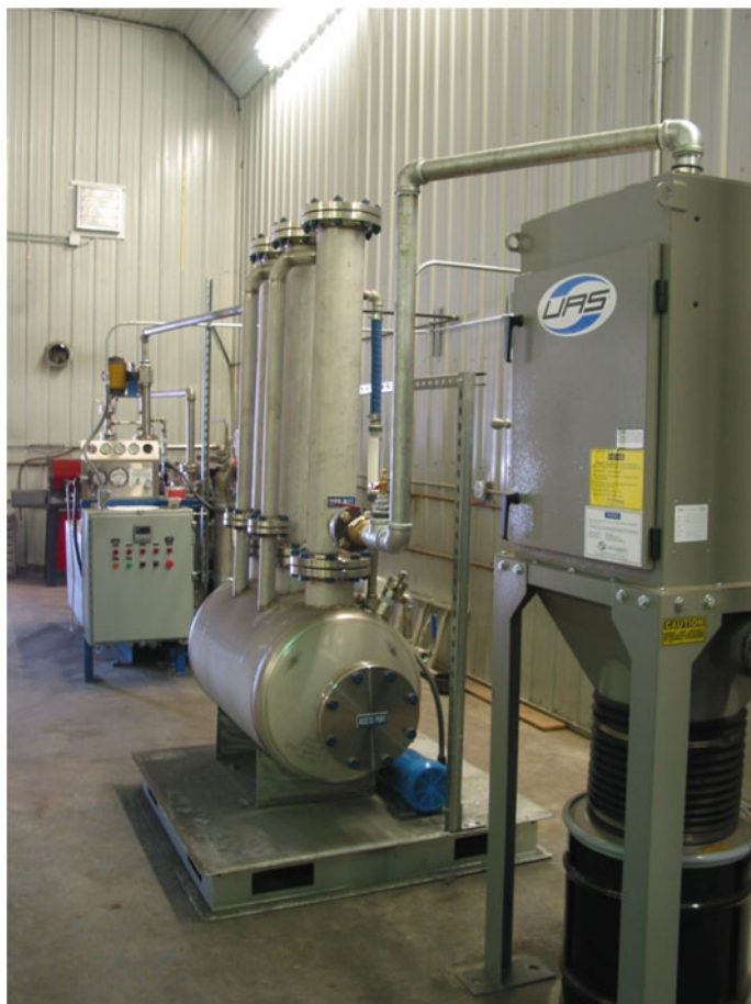
Fig. 11 The syngas treatment system comprising a bag house, a H_2S scrubber and a syngas compressor. (Color figure online)
