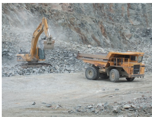
■ Fig. 2.9 Loading aggregates in a crushed stone (andesite) quarry for aggregates. (Image courtesy of Benito Arnó e Hijos, S.A.U.)
