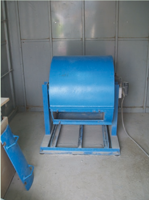
► Fig. 2.48 Steel drum in Los Angeles abrasion test
