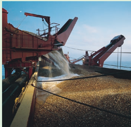
■ Fig. 2.6 Dredged material being transferred into the hold of the vessel. (Image courtesy of BMAPA)
