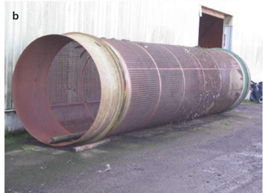
■ Fig. 2.32 Trommel (a) and the screen inside the device (b)
