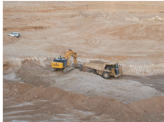
■ Fig. 2.15 Earthmoving machinery extracting sand and gravel aggregate
