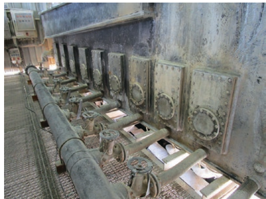
■ Fig. 2.35 Hydraulic classifier. (Image courtesy of SAMCA)
