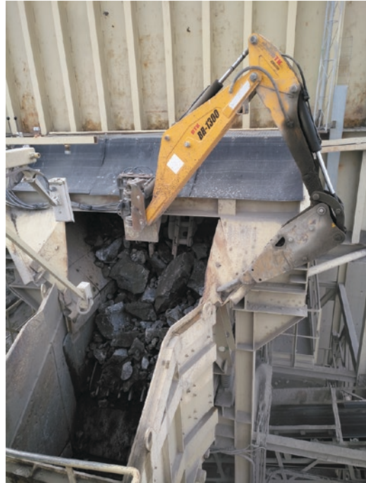
■ Fig. 2.23 Hydraulic hammer for crushing large pieces of rocks. (Image courtesy of Benito Arnó e Hijos, S.A.U.)
