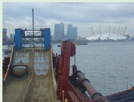
■ Fig. 2.7 Dredger unloading its cargo of marine aggregates close to the center of London with the use of scraper buckets. (Image courtesy of Mark Russel—BMAPA)
