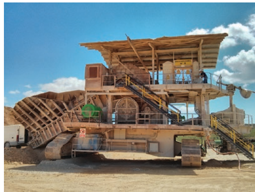
■ Fig. 2.24 Mobile crusher on the quarry floor. (Image courtesy of Octavio de Lera)
