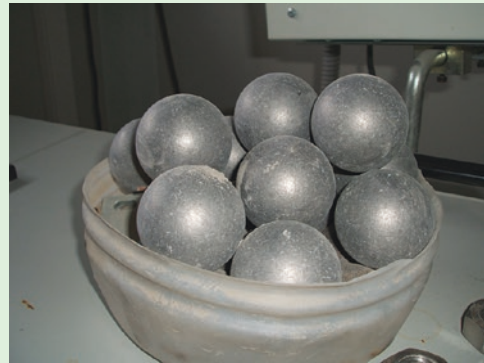
► Fig. 2.49 Steel balls in Los Angeles abrasion test
