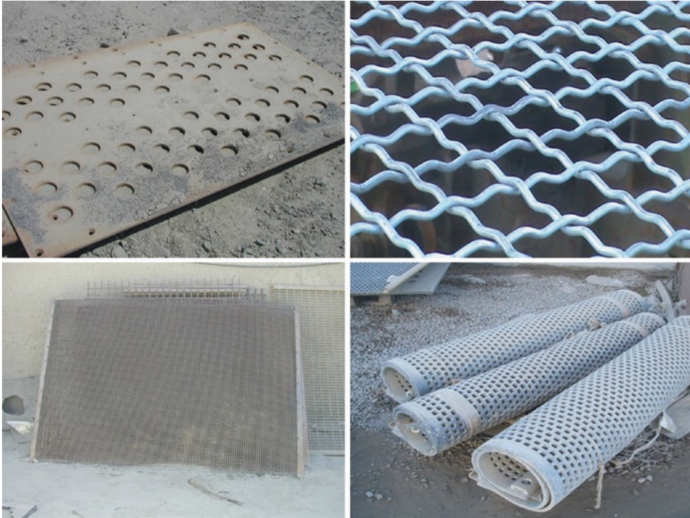
■ Fig. 2.33 Different types of screening surfaces and apertures
