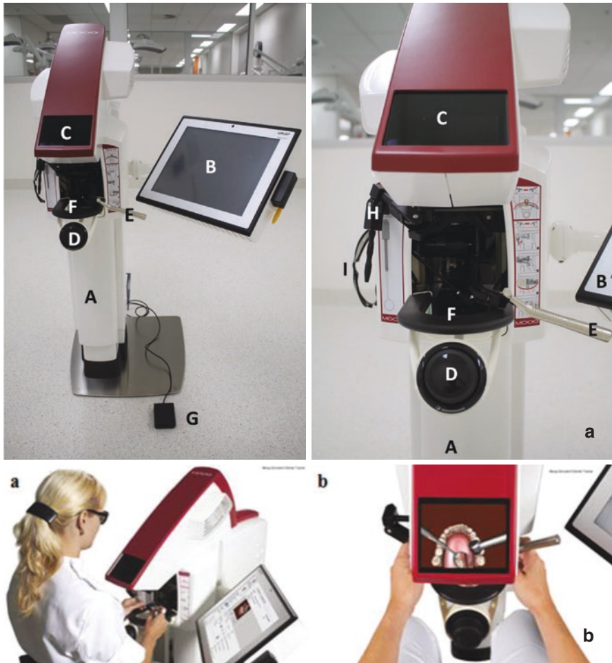
Fig. 14.4 (a) MOOG Simodont Dental Trainer showing different components (A) Simulator, (B) Screen, (C) Projection, (D) Space mouse, (E) Handpiece, (F) Hand rest, (G) Foot Pedal, (H) Mirror stick, (I) 3D Glasses (adopted from www.moog.com )). (b) A haptic tooth preparation exercise
