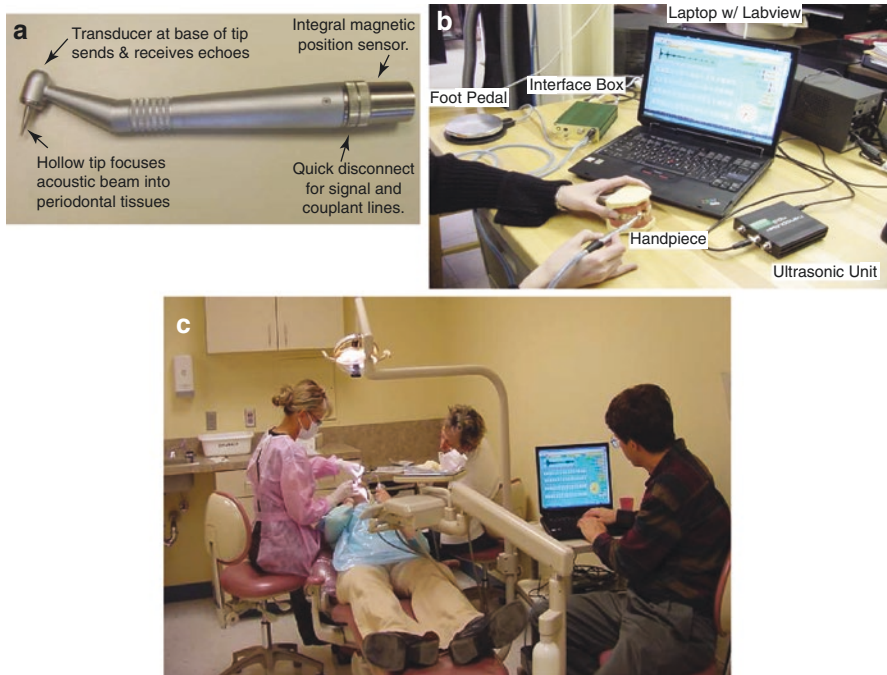
Fig. 2.10 (a, b) Ultrasonic Periodontal probe. (c) Investigational version of an ultrasonographic periodontal probe in a study performed in Norfolk, VA ( Courtesy of Prof. Mark K. Hinders )
