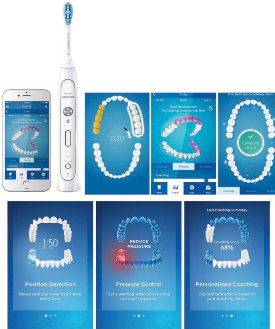
Fig. 1.1 Smart toothbrush and its working
