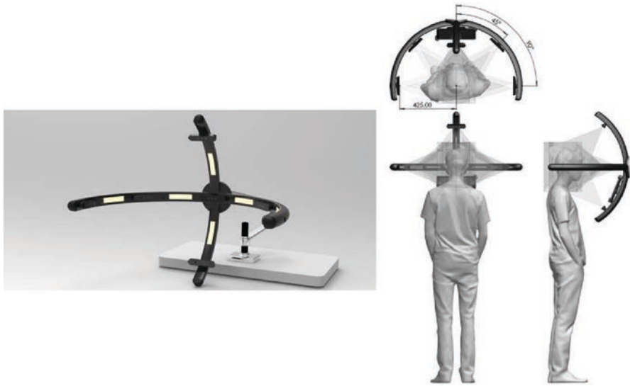
Fig. 7.5 Facial scanner (Adopted from https://www.bellus3d.com/arc )
