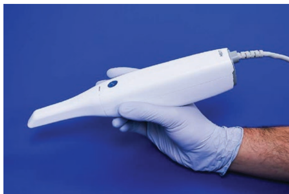
Fig. 6.13 Medit i500 scanner (Courtesy Dr. Ahmad, Institute of Digital Dentistry, NZ)
