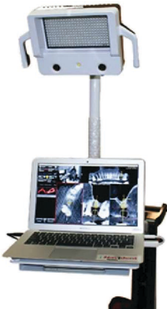
Fig. 4.19 Navident unit used for dynamic navigation (ClaroNav, Toronto, Canada)
