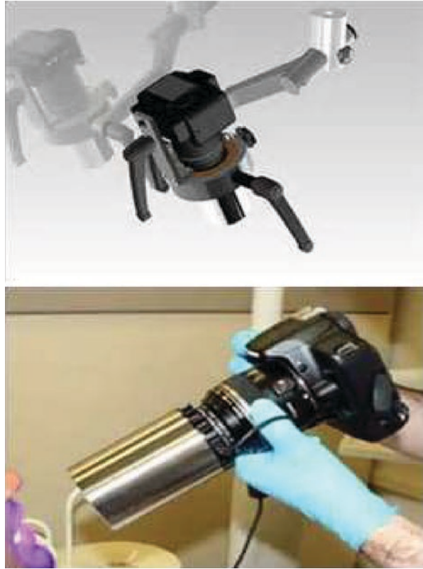
Fig. 2.3 The Inspektor™ QLF-D Biluminator™ 2+ camera system (Courtesy of Dr. Elbert de Josselin de Jong and Dr. Elbert Waller, Inspektor Research Systems, BV in Amsterdam, The Netherlands)
