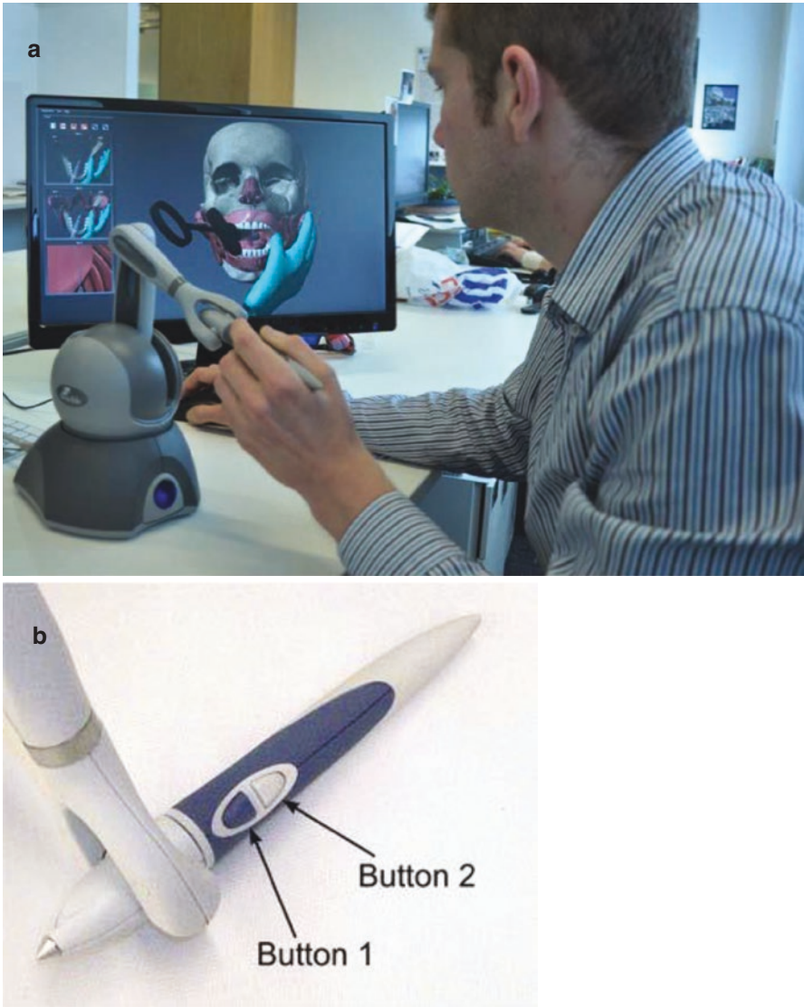
Fig. 14.5 (a) Haptic interaction for training the injection of a local anaesthetic [32]. (b) The two PHANTOM Omni pen buttons: one is for injection, and the other for reset
