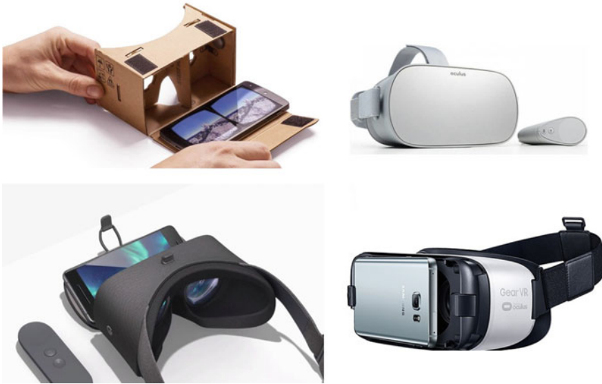
Fig. 1 HMD virtual reality devices, Google Cardboard (upper-left), Oculus Go (upper-right), Google Daydream (lower-left), GearVR (lower-right)
