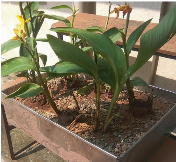
Fig. 3 Pictorial view of laboratory scale constructed wetland MFC during initial stage of construction
