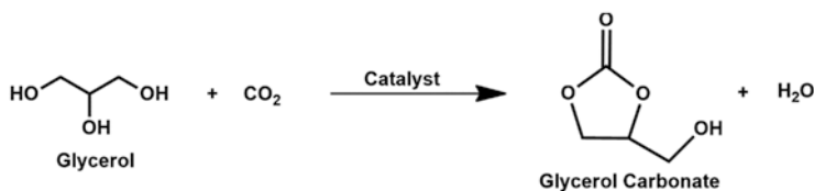
Scheme 8 Synthesis of glycerol carbonate from glycerol by direct carboxylation with carbon dioxide
