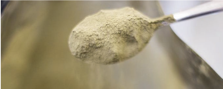
Fig. 4.2 Locally produced protein powder made from the juice of a screw press processing in the Green Grass Biorefinery. Production of the feedstock, perennial green grass or clover grass, as compared to growing, e.g. cereals, has an environmentally friendly profile: it can be cultivated without the use of pesticides, and it gives (under Danish conditions) twice as much biomass and only half the run-off of surplus nutrients per hectare. (Photo: Ida Marie Jensen, Aarhus University, Denmark)
