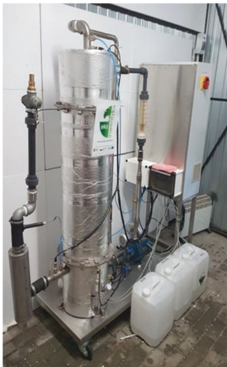
Fig. 17.3 Laboratory setup including small-scale CTBB. (Ekoinwentyka Ltd.)
