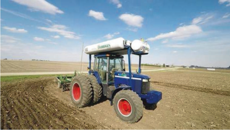
Fig. 15.9 The solar hydrogen ammonia tractor. (Photo courtesy of Jay Schmuecker)
