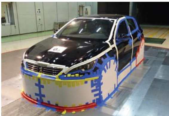
Fig. 9 Vehicle in the wind tunnel fitted with sleeve
