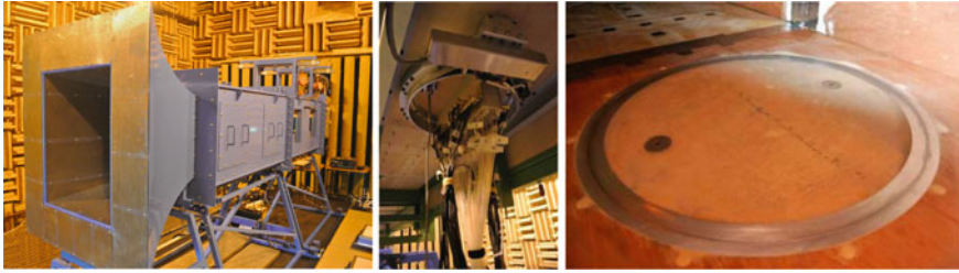
Fig. 6 Different views of the SONOBL set-up; at left, overall view of the wind tunnel inside ECLyon anechoic room; at right, a photo of the rotating disk supporting B&K microphones and a line array of 63 irregularly distributed remote microphones; in the center, a bottom view of the disk is shown and the tubing used to eliminate any reflective waves is apparent
