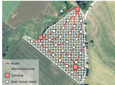
Fig. 6. Intended network topology at one of the test sites in Brandenburg
