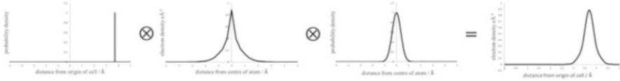
Fig. 2 The convolution of atom position, atomic scattering density and displacement term give the overall atom scattering density
