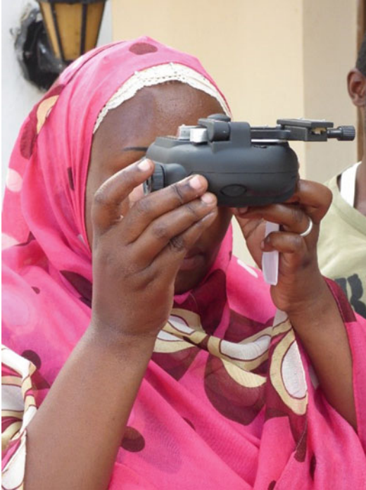
Fig. 5 Microscopy in the field. A range of microscopes can be employed successfully in locations where there is no electricity, including older styles that are equipped with mirrors. Here a battery-operated handheld Newton Microscope is used by a local member of the community on the Coast of East Africa
