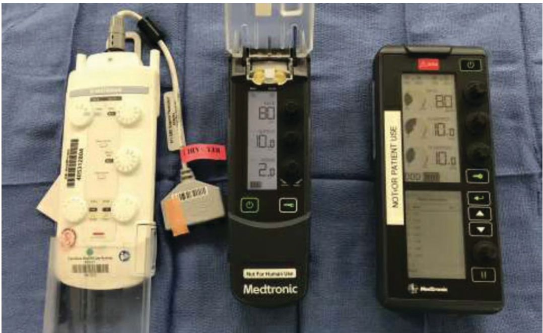
Fig. 18.3 Transvenous pacing boxes. The first two are single chamber and the third (right) is dual chamber
