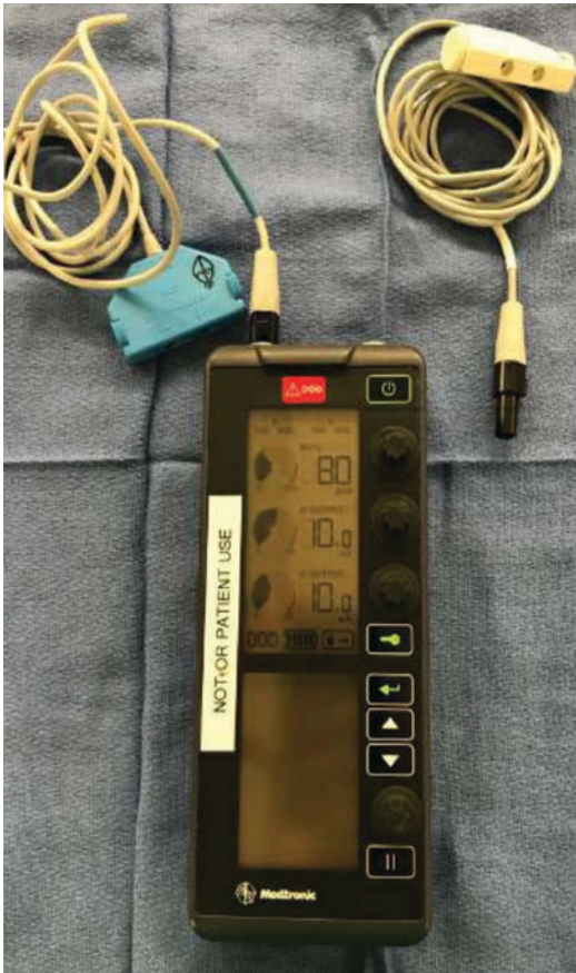
Fig. 18.5 Dual-chamber temporary pacemaker box, epicardial atrial connector on the left, ventricular connector on the right
