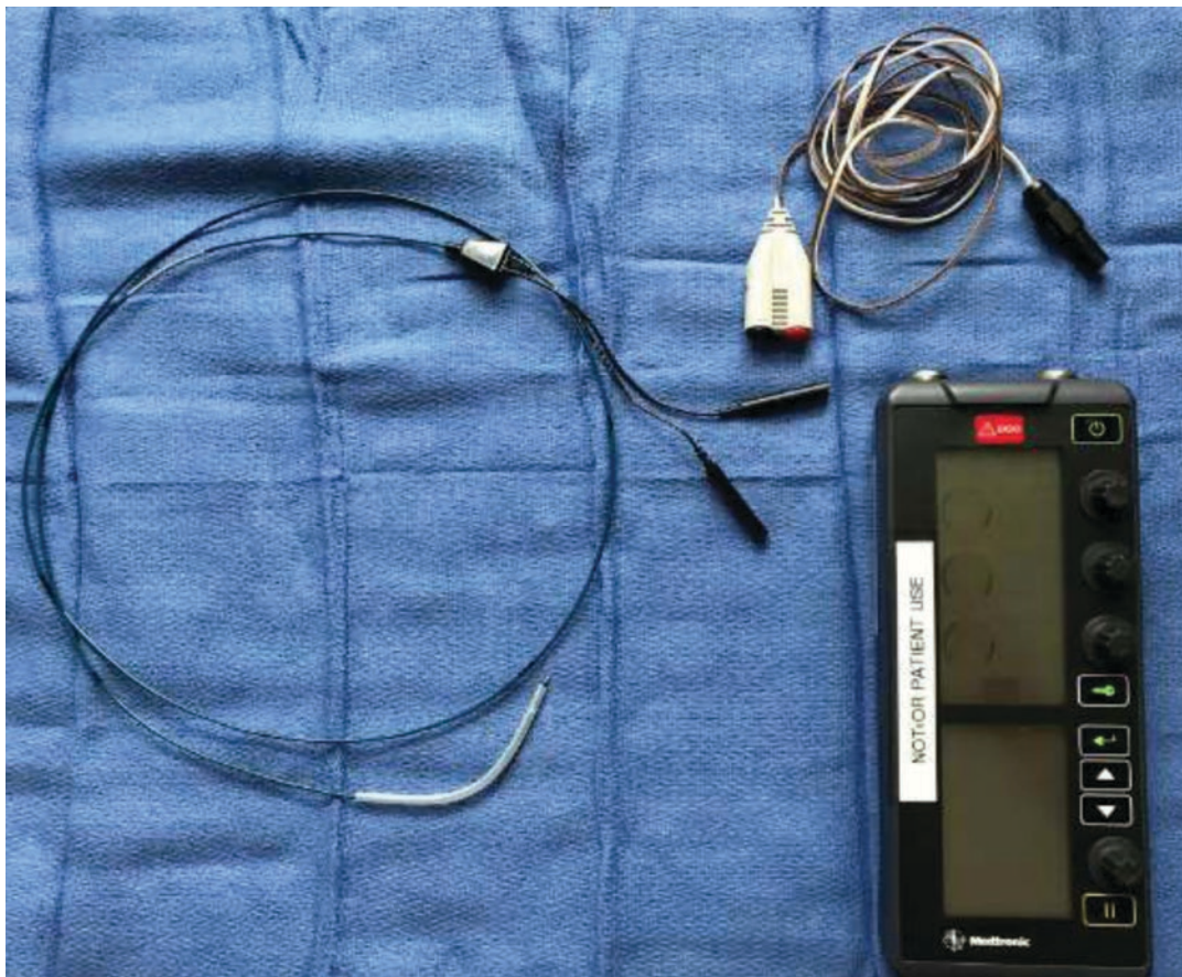
Fig. 18.6 Temporary transvenous pacing wire on the left. The upper right is the connector. Temporary pacing box is on the lower right.
