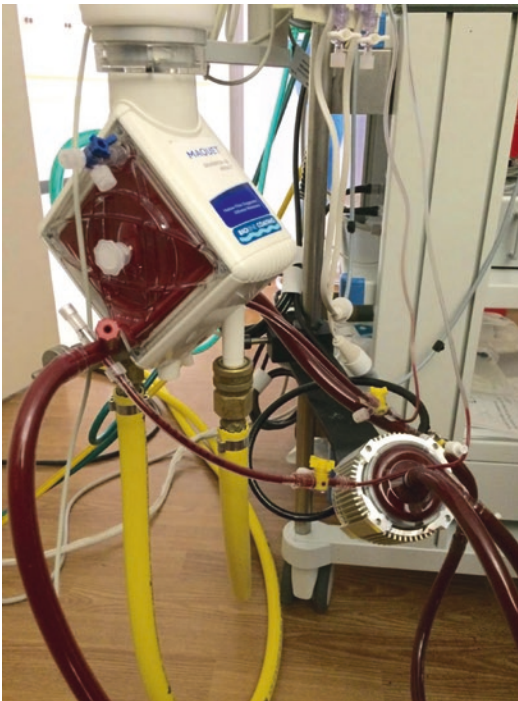
Fig. 21.4 ECMO circuit: Top left: membrane oxygenator, oxygenates blood and removes CO 2 as blood passes through it. Bottom right: centrifugal pump, pumps blood through the circuit using a rotating impeller that spins creating negative pressure in the pump head
