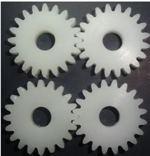
Fig. 2.6 Involute (above) and S-gears (below) made of PA66 (left) and POM-C (right)
