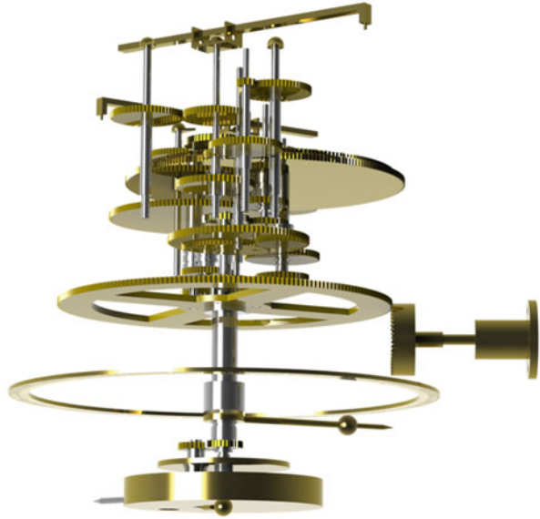
Fig. 9.5 The Antikythera mechanism, 3D model of the inner structure
