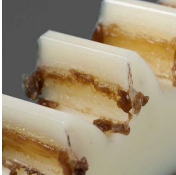
Fig. 4.1 Melting damage at PA12 gears [3]
