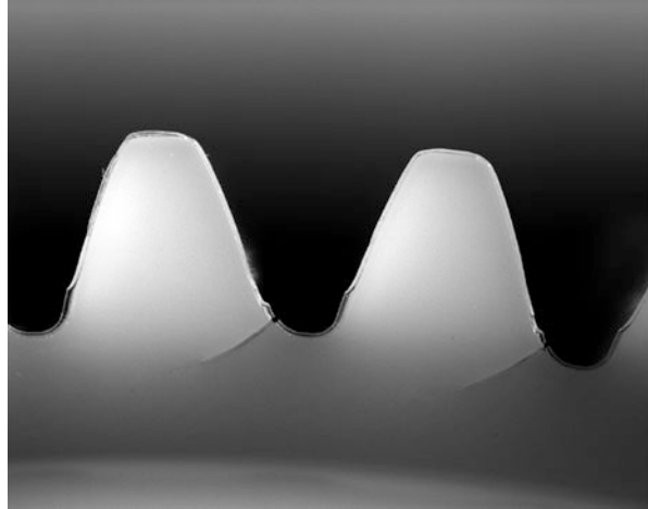
Fig. 4.16 Exemplary tooth root fracture of a KST-B POM gear [10]
