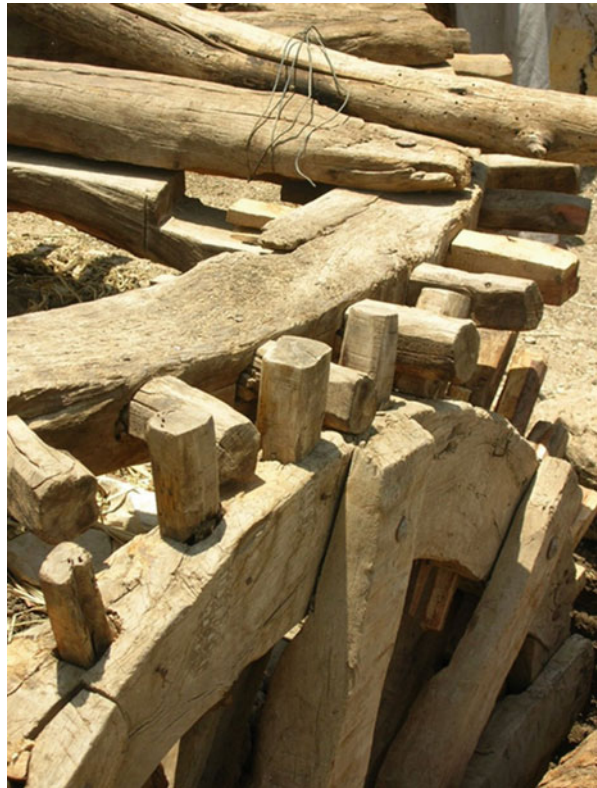
Fig. 9.2 Gearing of a sakia [1]
