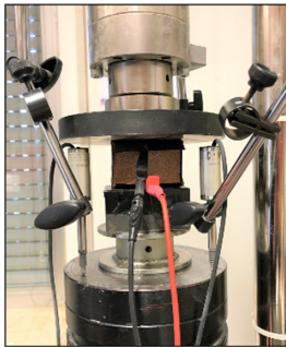
Fig. 2. Testing setup and load history adopted to perform axial compression tests on single smart bricks instrumented with a couple of traditional strain gauges.
