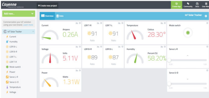
Fig. 12 IoT monitoring application of solar tracker system
