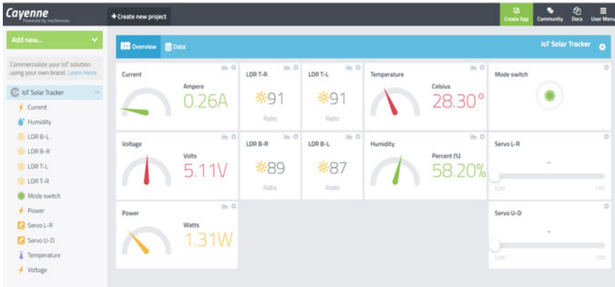
Fig. 12 IoT monitoring application of solar tracker system
