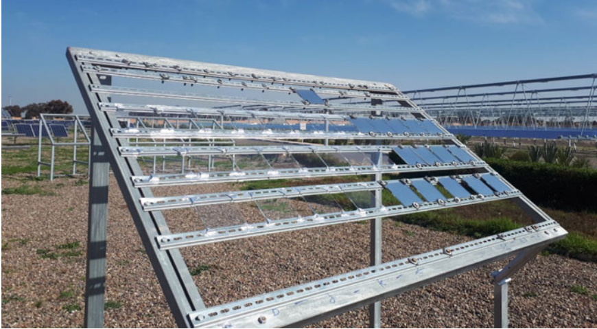
Fig. 5 Glass samples were exposed in the fixed rack at the Green Energy Park research facility
