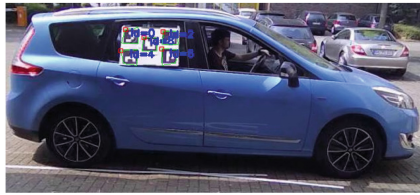
(b) ArUco markers detected by Marker-based Estimator.
