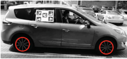
(a) Wheels detected by Wheel Detection Estimator.
