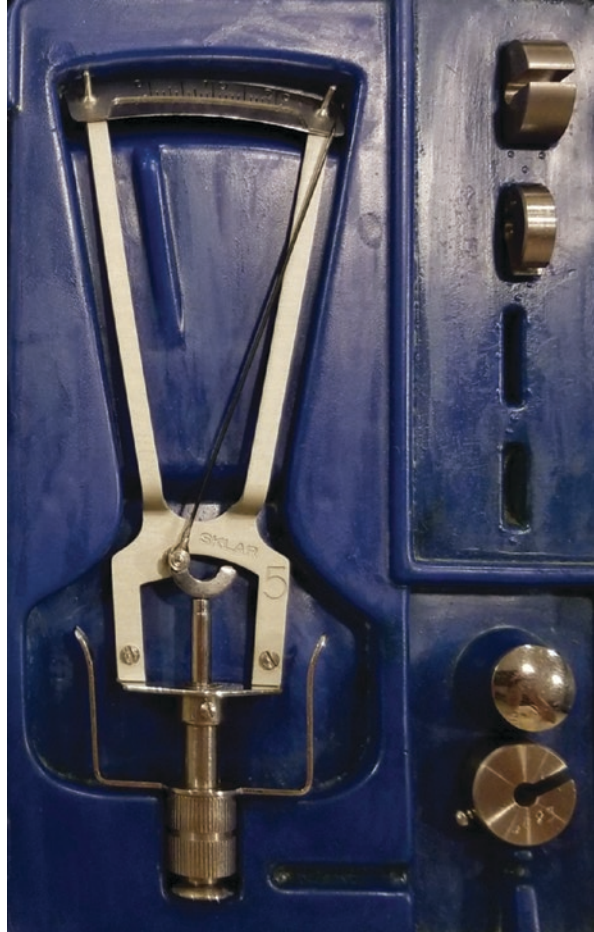
Fig. 13.1 Schiøtz tonometer with different weight attachments
