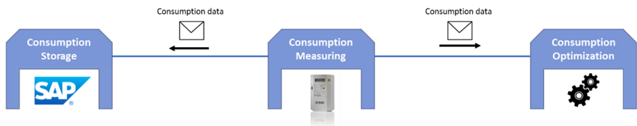
Fig. 6. State of the I4.0 system configuration after matching the components “Consumption Measuring” and “Consumption Optimization”
