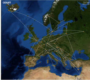
(a) GEANT Topology. 13 producers, 8 consumers, 32 routers acting as in-network caches. From the Internet Topology Zoo[13]. Figure from http://www.topology-zoo.org/dataset.html
