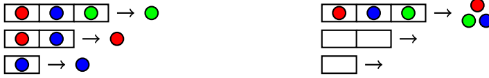
Fig. 4. Examples of valid sets of IS outputs. On the left, we have the “ordered” execution in which every process outputs a distinct set of inputs (blue - only itself, red - blue and itself, and green - all three). On the right, we have the “synchronous” execution in which all three processes output all the inputs. (Color figure online)
