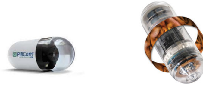
Fig. 2.2 Illustration of (left) PillCamSB3 and (right) Capsovision WCE with a lateral sensors for non-conventional image acquisition of the small intestine. Respectively taken from VideoDigest2017 and www.ortoday.com
