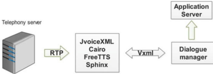
Fig. 1 Spoken dialogue system architecture
