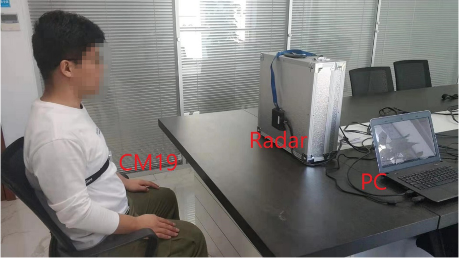
Fig. 5. Photograph of the experiment of human vital signal detection
