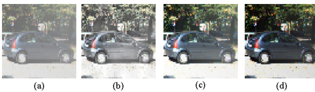
Fig. 10. Comparison of fogging effect at high fog concentration: (a) high fog concentration image (b) adaptive histogram equalization algorithm (c) single-scale Retinex algorithm (d) dark channel prior algorithm
