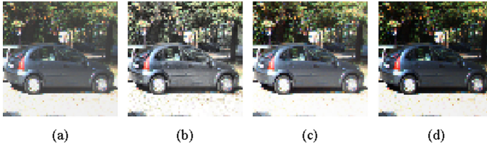
Fig. 8. Comparison of fogging effect at low fog concentration: (a) low fog concentration image (b) adaptive histogram equalization algorithm (c) single-scale Retinex algorithm (d) dark channel prior algorithm
