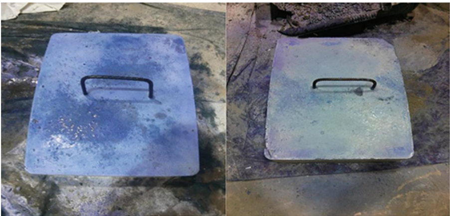
Fig. 5. (a) Concrete without \text{TiO}_2 and (b) Concrete with \text{TiO}_2
