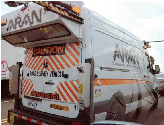
Fig. 2. ARAN truck for roadway and bridge deck scanning
