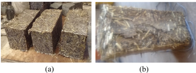
Fig. 4. Wheat straw saw dust block blocks (a) and respective failure pattern (b)
