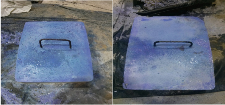
Fig. 4. Specimens with permanent blue Meltheylene dye
