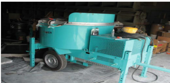
Fig. 1. High-energy paddle mixer for developing SCC mixes
