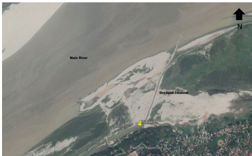
Fig. 21.4 Satellite imagery of the dredged channel (2019) constructed after conducting the model study which shows the flow of water in the channel passing through the intake point
