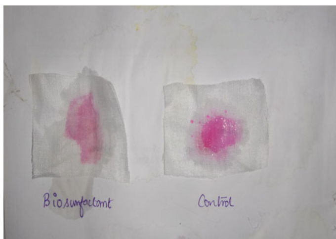
Fig. 11 Picture showing the efficacy of biosurfactant as stain removal of azo dye
