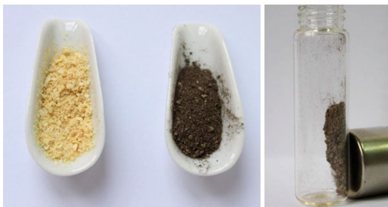
Fig. 8.2 Native and magnetically modified orange peel (left) and magnetic separation of magnetically modified biosorbent (right). Magnetic modification was performed by indirect postmagnetization procedure employing magnetic iron oxide nano- and microparticles prepared by microwave-assisted synthesis from ferrous sulfate at high pH
