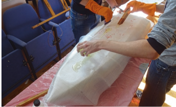
Fig. 8.2 Hull covering by fiberglass
