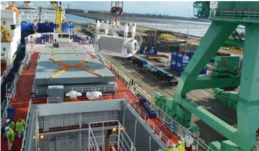
Fig. 20.3 Unloading cask with nuclear cargo from PNTL ship's hull. (Source: [13])
