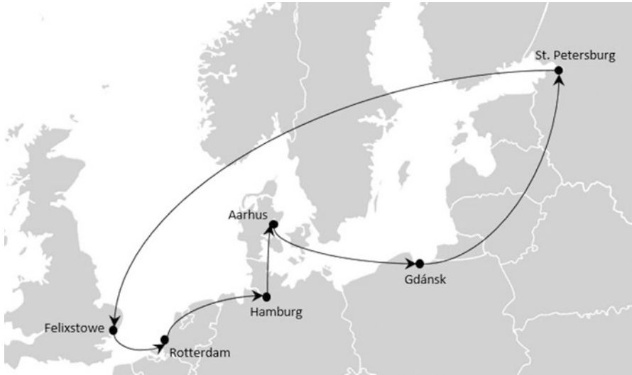
Fig. 15.3 Example of a simple service, where each port is visited exactly once
